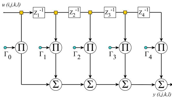
Fig. 4. First-order 4D FIR direct-form digital filter
