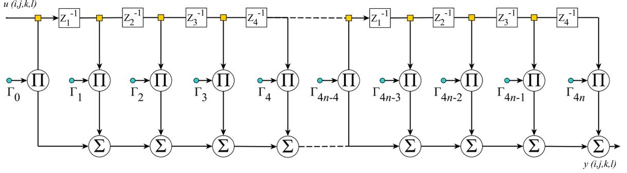
Fig. 3. Generalized 4D FIR direct-form digital filter
